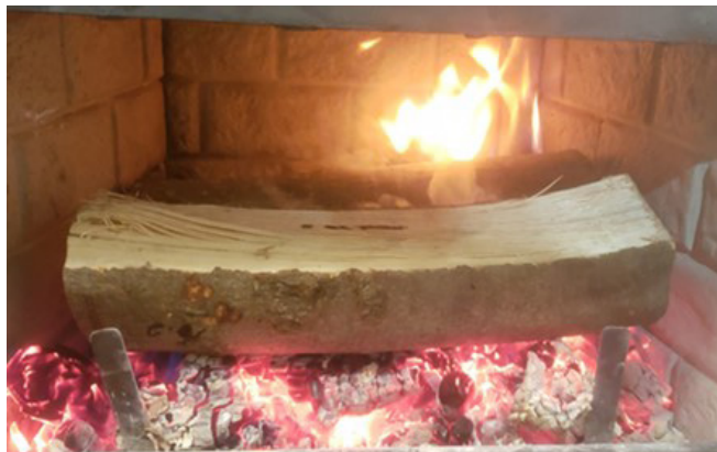
Figure 25: Maintenance-fire load in firebox
