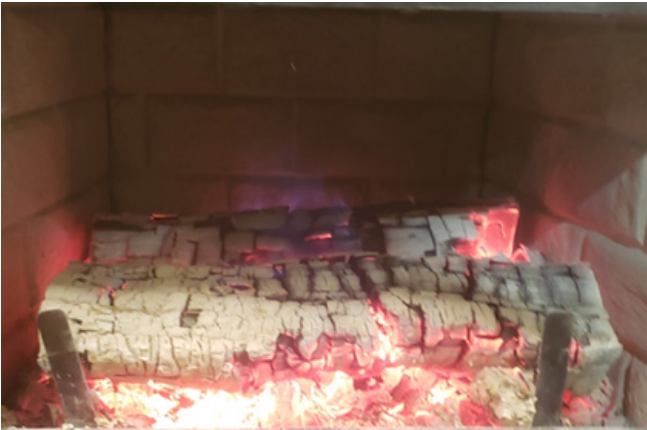
Figure 28: Charcoal bed at the end of Maintenance-fire phase
