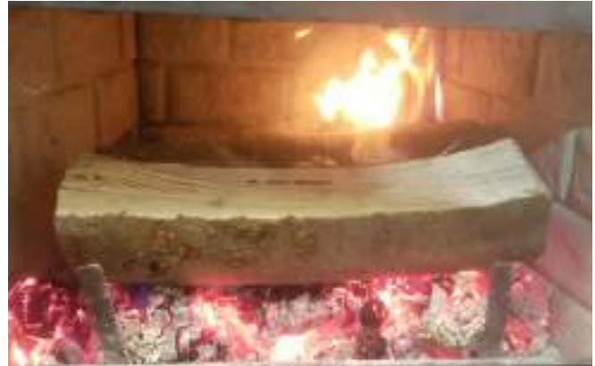
Figure 26: Maintenance-fire load in firebox
