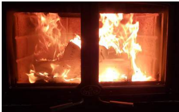
Figure 19: Flames intensity at the beginning of Start-up phase (Door cracked about 1 inch)
