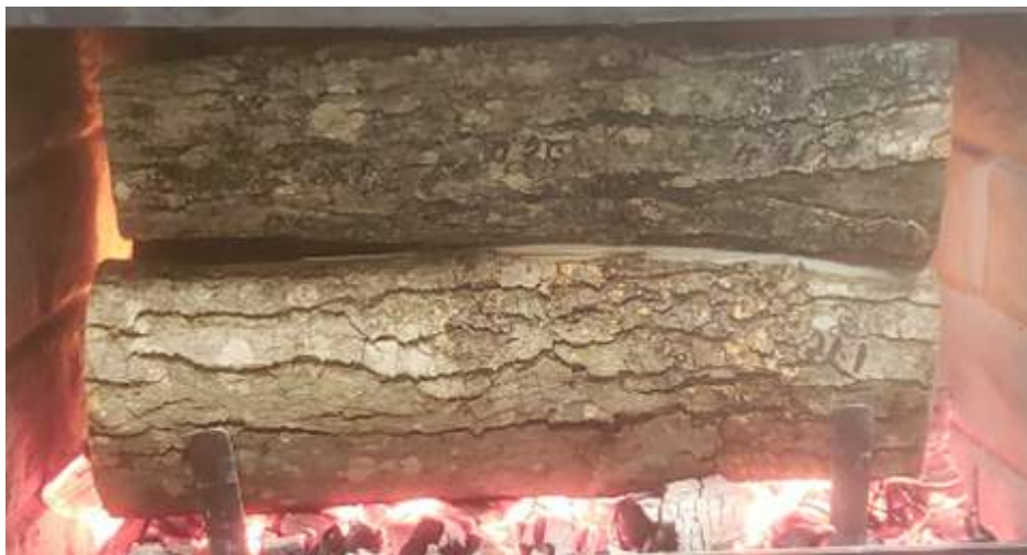
Figure 31: Low-fire load in firebox
