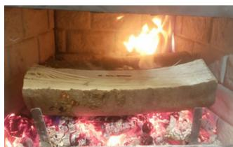
Figure 24: Charcoal bed at the end of High-fire phase
