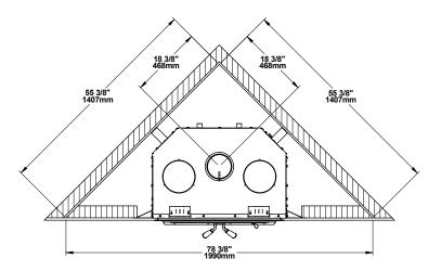
Framing configuration should be used as a reference only. If a finishing material is installed inside the enclosure, its thickness must be added to the following measurements. Theses values are minimum measurements and may need to be increased to allow the installation of the fresh air intake, the forced air kit or the type of finishing material used.
