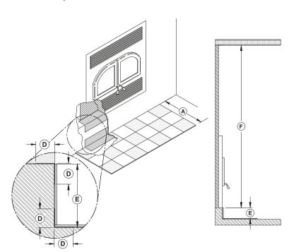
When the fireplace is installed on a raised base of 4" (101 mm) or more **(E)**, a non-combustible floor protection of at least 16" (406 mm) **(A)** with no R value, must be installed in front of the fireplace.
