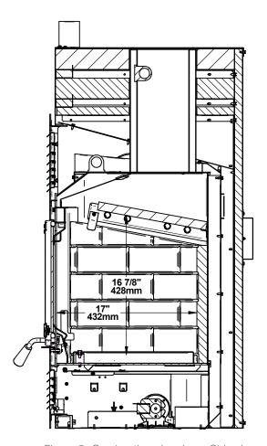
Figure 8: Combustion chamber - Side view
