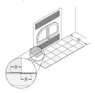
When the fireplace is installed directly on the floor, a non-combustible floor protection of at least 16" (406 mm) (A) with an R value of 1.00 must be installed in front of the fireplace. The joint between the floor protection and the fireplace must be protected over the entire width of the floor protection by a folded and continuous metal sheet (D = min 2" [51 mm]) (not supplied).
