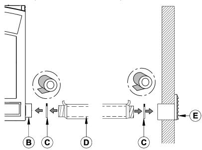
7. To complete the installation, make a hole of ¼" to ½" (6 mm to 13 mm) bigger than the duct diameter on the outside wall of the house at the chosen location. From outside, place the outside wall register in the hole (open side down) and fasten the register to the wall, with screws.
