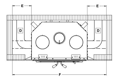
If a finishing material is installed inside the enclosure, its thickness must be added to the following measurements.
