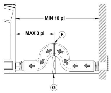
It is mandatory to install a mechanical shutter, right or left side depending on the installation of the air intake, that closes the outside air inlet when the fireplace is not in use.
