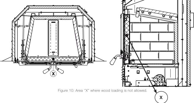
The overall firebox calculation is an approximation and is not intended to be used for loading. This volume includes a buffer zone to allow an easier fuel insertion, prevent ash spillage and allow the air wash to work properly.
