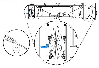
5. Install the hatch **(A)** supplied with the product, with the hardware **(B)** provided in the manual kit.
