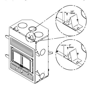
Do not use combustible materials for the frame directly above the fireplace. This area should remain empty to a height of 80" (2032 mm) measured from the base of the fireplace.
