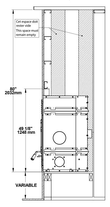
If a finishing material is installed inside the enclosure, its thickness must be added to the following measurements.
