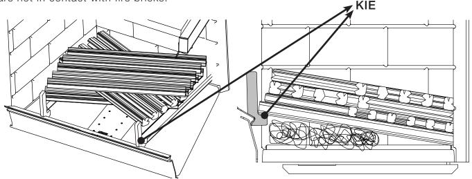
Figure 13: Kindling configuration using Kindling Ignition
