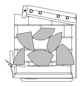
Figure 27: Low-burn rate load configuration - Side view
