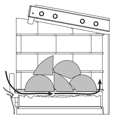
Figure 21: Air path under the High-fire load
