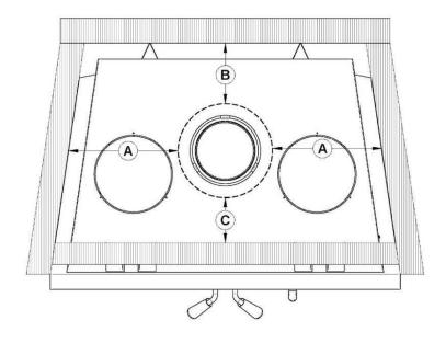
For example, for the next installation, the chimney cannot be closer to the combustible materials than the **value (A)**. Therefore, the enclosure should be 11 inches (27,94 cm) from the chimney.
