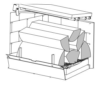
Figure 26: Low-burn rate load configuration - Top view
