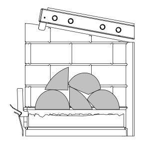
Figure 19: High-fire load configuration with medium size wood pieces
