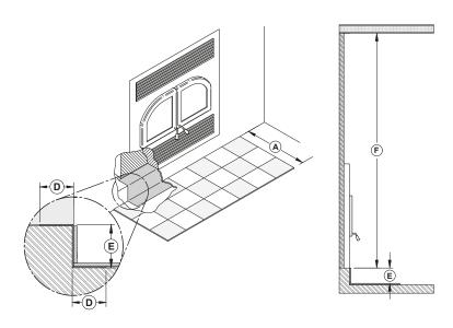
When the fireplace is installed on a raised base of less than 4" (101 mm) **(E)**, a non-combustible floor protection of at least 16" (406 mm) **(A)** with an R value of 1.00 must be installed in front of the fireplace.
