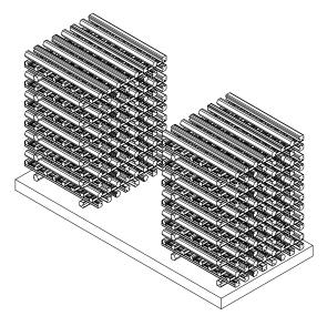
Figure 15: Kindling pieces in a criss-cross stack
