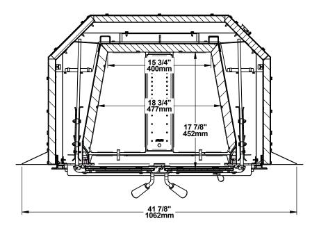
Figure 6: Combustion chamber - Top view
