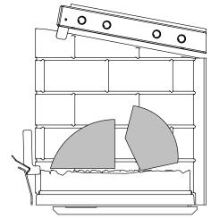
Figure 23: Maintenance-fire load configuration - Side view
