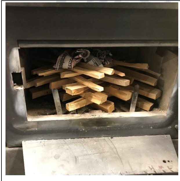
Kindling & Start-up Loaded in Stove
