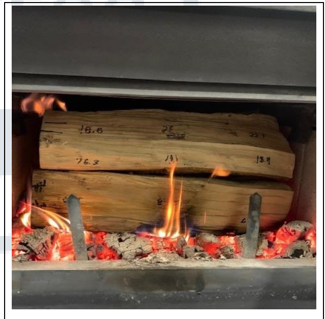
Medium Fire Fuel Loaded
