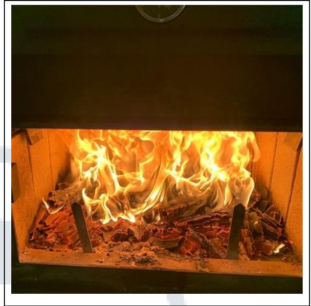
Residual Start-up Fuel Coal Bed – Post Rake
