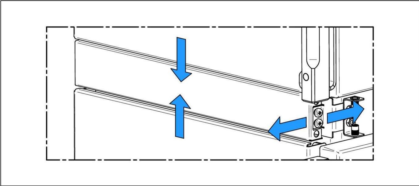
**3** - Secure the central molding (C) with screws (I) once the adjustment is complete. Press firmly on the central molding against the side moldings while tightening the screws.
