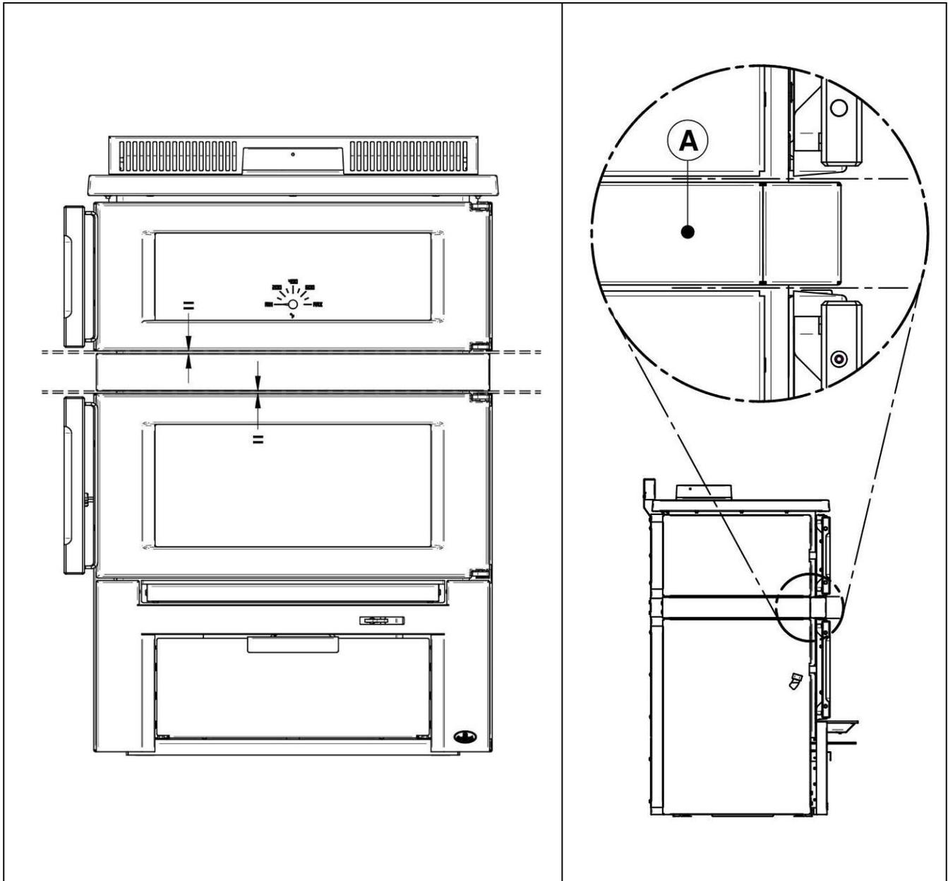
\* It may be necessary to readjust the doors to straighten them and achieve perfect alignment. (Refer to the product manual for adjustment.)
