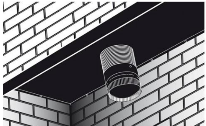
Figure 29: Plaque non combustible
