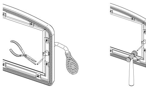
Figure 23: Removing the split pin
