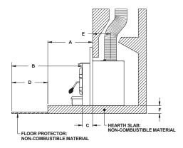
Figure 31: More than 5" raised base installation
