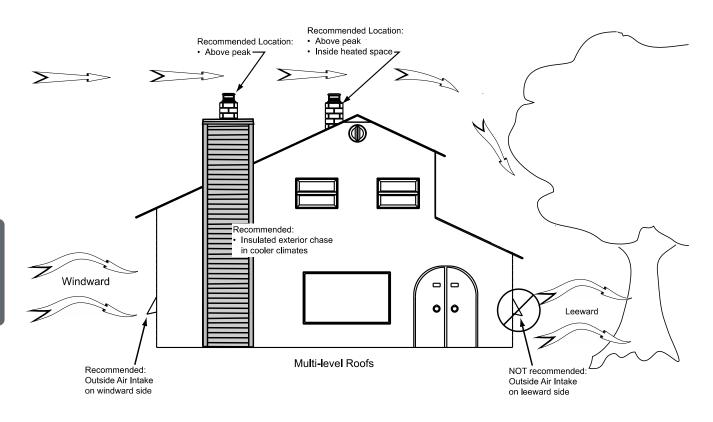
Figure 42: Air supply in conventional houses
