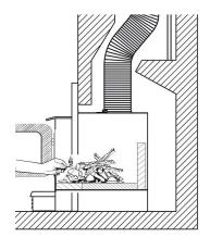
stacking). Open the air intake control completely and light the newspaper. The free flow of flames around each piece of wood and the absence of smoke indicate a quality ignition. Leave the door slightly ajar for about 5 minutes. When the fire is well lit, close the door while keeping the air intake control open. When the small kindling wood is almost completely burned and the medium-sized pieces are still burning, it's time to add larger pieces of wood until the fire is well established.
