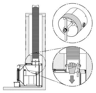
Figure 37: Liner fastening system
