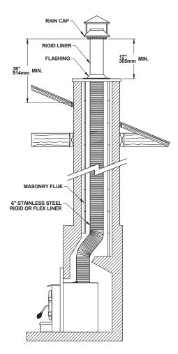
Figure 35: Liner Installation
