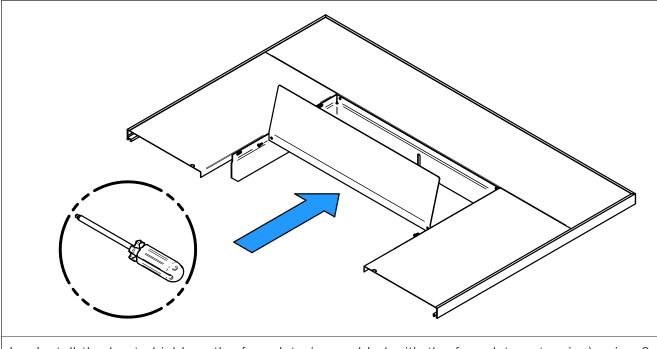
1. Install the heat shield on the faceplate (assembled with the faceplate extension) using 3 selfdrilling screws included in the kit. The heat shield should be pointing upwards.
