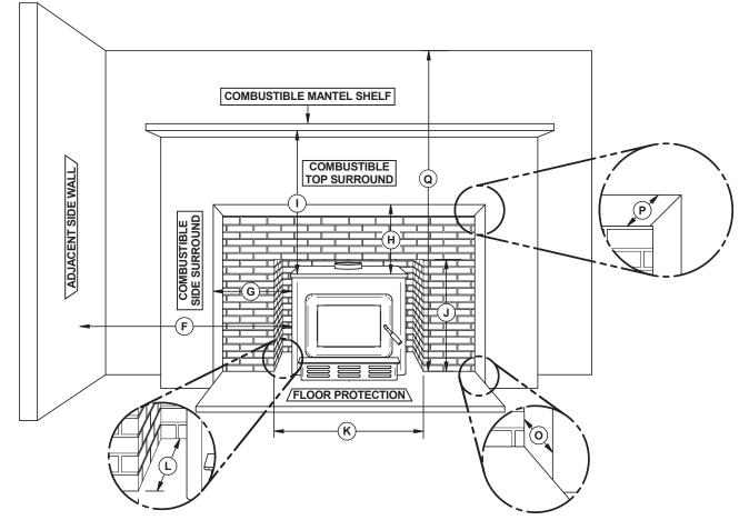
Figure 32: Masonry Opening and Clearances
