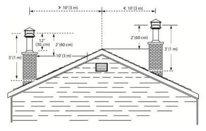
Figure 40: Minimum Chimney Height
