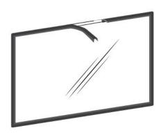
Do not over-tighten the screws. Note that the two main causes of broken door glass are uneven placement in the door and over-tightening of retaining screws.
