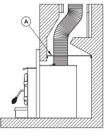
Figure 33: Block-off Plate
