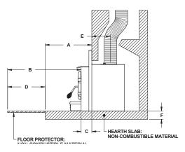
Figure 30: 5" or less raised base installation
