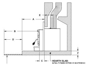
Figure 29: Additional Floor Protection
