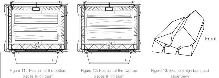
For optimal loading of a high fire, take small to medium size fuel pieces (between 2- and 3-inches cross section dimensions approximately) on the bottom and use medium to large size fuel pieces (3.5 to 4.5 inches of cross section dimensions approximately) on top. To make sure combustion is equal, put the biggest piece on top of the first three, at the front of the firebox. See an example of high burn load in the Figure 13 above.
