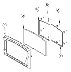
Figure 25: Replacing the glass
