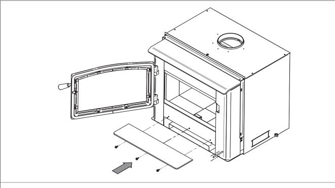
1. Before installing the blower, open the door and install the ash lip by screwing it in place with 3 screws, located in the user manual kit.
