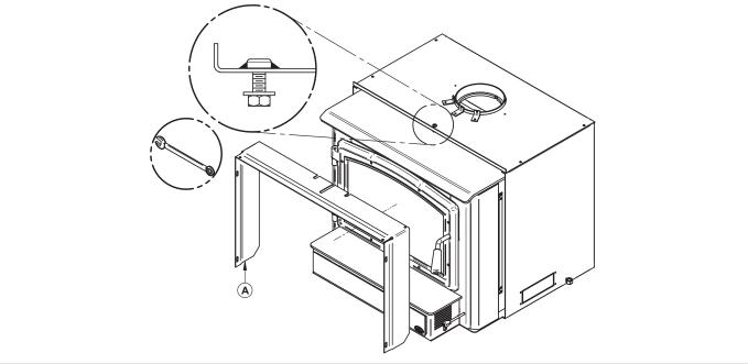
1. Remove the faceplate extension (A) secured between the firebox and the convection air jacket.
