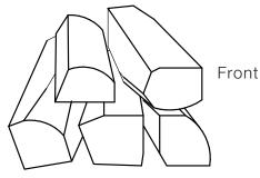
Figure 14: Position of the bottom pieces (Low burn)
