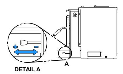
Figure 22: Air Supply Control
