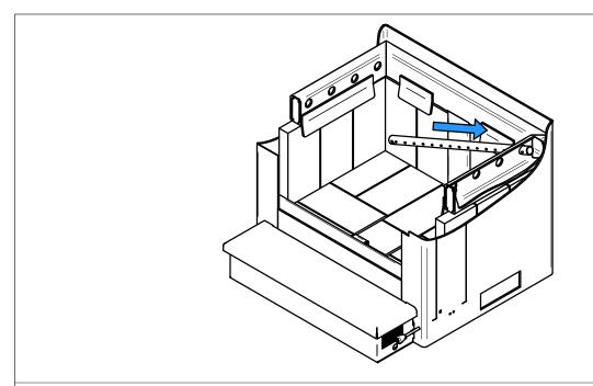
1. Starting with the rear tube, lean and insert the right end of the secondary air tube into the rear right channel hole. Then lift and insert the left end of the tube into the rear left channel.
