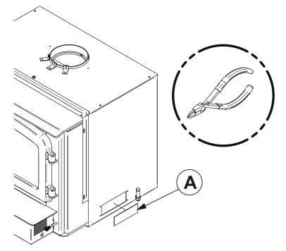
1. Using pliers, remove the rectangular metal plate (A) retained by the micro-seals to clear the opening for the outside air intake.
