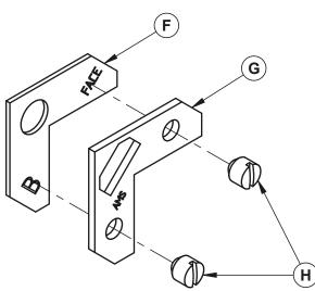
Partially thread the screws (H) on the trim's 4. corner bracket (G) then superimpose the corner brackets (F) and (G) as shown.
