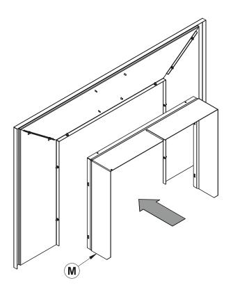
7. Align the holes in the faceplate extension (M) with the holes in each faceplate side panels.
