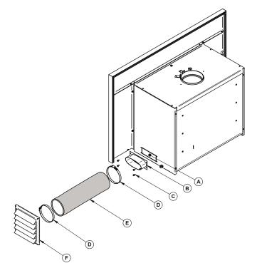
Install the fresh air intake adapter (B) with four screws (C) then secure the flexible pipe<sup>19</sup> (E) (not included) to the adapter (B) using one of the pipe clamps (D). Secure the other end of the pipe to the outside wall termination (F) using the other pipe clamp (D). The outside wall termination (F) must be installed outside of the home.
