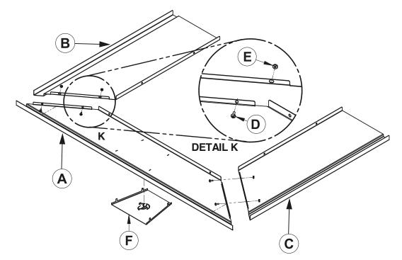
Place the faceplate panels with the finished side down on a flat, soft, non-abrasive surface. Line up the holes of the upper faceplate panel (A) with the holes of the side panels (B) and (C). Secure them together using four bolts (D) and nuts (E) provided. Insert the plate (F) in the slots at the center of the upper faceplate panel (A).
