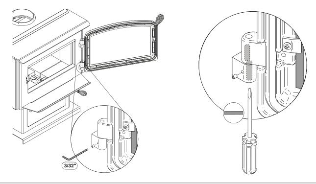
Using a flat screwdriver, turn the adjustable hinge rods in the direction shown to adjust the doors. Tighten all door hinge pressure screws when they are at the desired positions. Configurations 1-2-3-4-5-6, show in which direction these act on the adjustment of the door.
