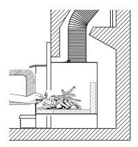
Do not leave the insert unattended when the door is slightly open. Always close and latch the door after the fire ignites.
