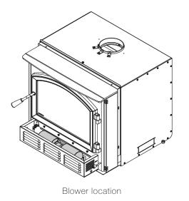
A blower is already installed on this insert. It is located underneath the ash lip, in front of the insert. Its function is to increase airflow through the heat exchanger and improve hot air circulation in the room. When used regularly, the blower can provide a small increase in efficiency, up to 2%. However, the use of a blower should not be used as a way to gain more output from an insert that is undersized for the space it is intended to heat.
