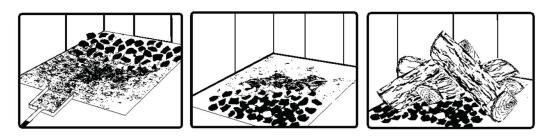
Raking the coals is useful for two reasons. First, it brings them near where most of the combustion air enters the firebox. This will ignite the new load quickly. Secondly, the charcoal will not be smothered by the new load of wood. When the embers are simply spread inside the combustion chamber, the new load smoulder for a long time before igniting.
