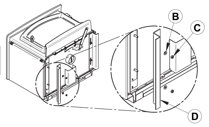
3. Install the pedestal (E) on the stove and screw it in place using washers (B) and nuts (C).
