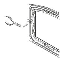
Figure 36: Removing the split pin
