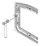
Figure 37: Installing the split pin
