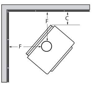
If the clearance reduction is on the same side as the door handle, position the stove at a minimum of 6 inches from the side wall (clearance B), otherwise it may be located at the clearance shown in the table above.
