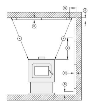
Figure 33: Heat shield clearances
