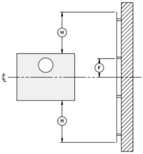
Figure 34: Heat shield clearances
