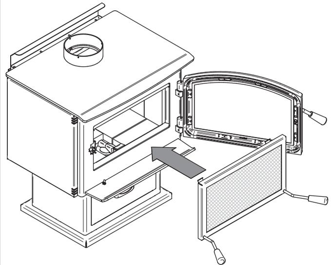
3. Lean the upper part of the fire screen against the top door opening making sure to stow the top fire screen brackets behind the primary air deflector.
