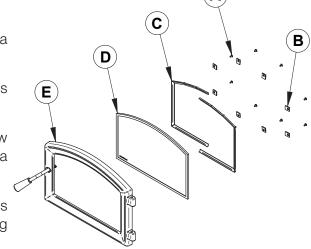
The two main causes of broken door glass are uneven placement in the door and overtightening the retaining screws.
