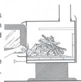
Once the fire has ignited, the door can be closed with the air control still fully open. When the kindling is almost completely burned, standard firewood pieces can be added.
