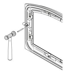
Figure 19: Installing the split pin
