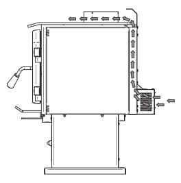
Figure 16: Air flow with a blower
