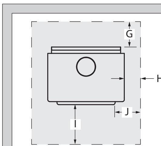
Figure 23: Protection de plancher
