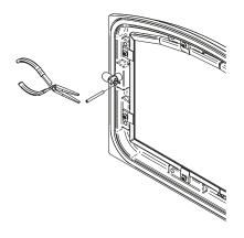
Figure 17: Removing the split pin
