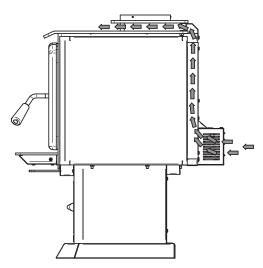
Figure 15: Air flow with a blower
