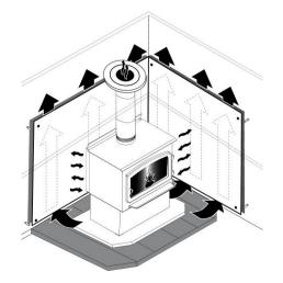
Figure 23: Heat shield
