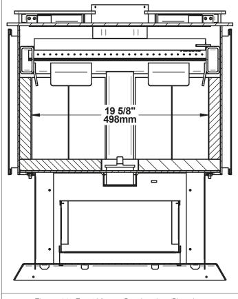
Figure 11: Front View - Combustion Chamber
