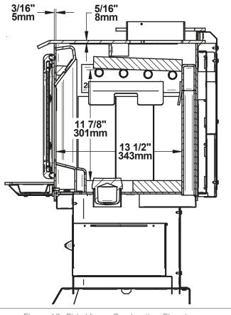
Figure 12: Side View - Combustion Chamber
