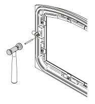
Figure 18: Installing the split pin
