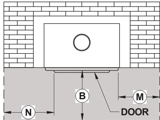
Figure 17: Protection de plancher
