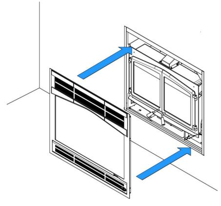
4. Attach the upper springs on the faceplate to hold it in place.
