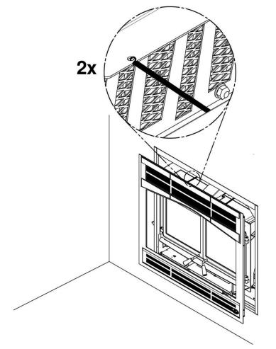
5. Firmly push the faceplate against the fireplace. Using a power driver, secure the bottom with 2 self-tapping screws (one on each side) provided with the fireplace owner's manual.
