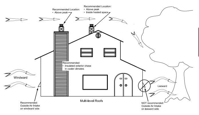
Figure 25: Air supply in conventional houses
