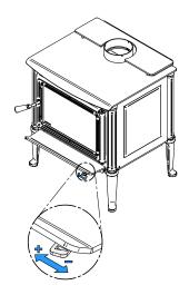
Figure 9: Air Intake Control
