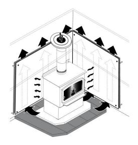
Figure 19: Heat shield
