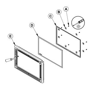
Figure 13: Replacing the glass
