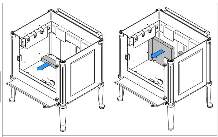
3. Remove the bottom bricks (2) at the back of the stove then remove the back bricks (6).
