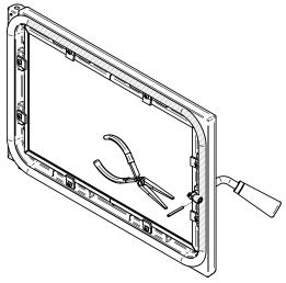
Figure 10: Removing the split pin
