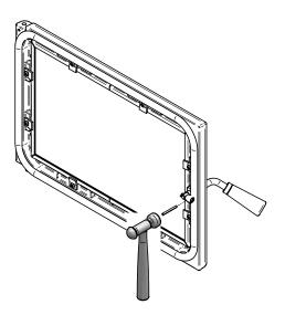
Figure 11: Installing the split pin
