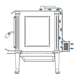
Figure 7: Air flow with a blower
