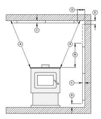
Figure 22: Heat shield clearances
