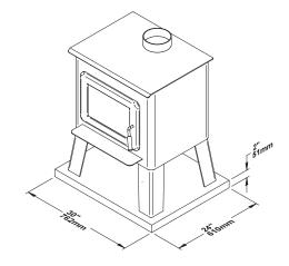
Figure 18: Floor protection in a mobile home
