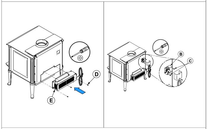
2. Screw the blower **(E)** in place using the screws **(D)** included in the installation manual. Screw the thermodisc **(B)** with the screws **(C)** supplied with the thermodisc on the back of the stove.
