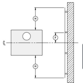
Figure 21: Heat shield clearances
