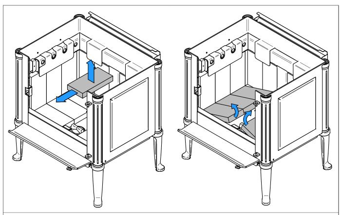
Remove the center floor brick and then remove the 6 other floor bricks.
