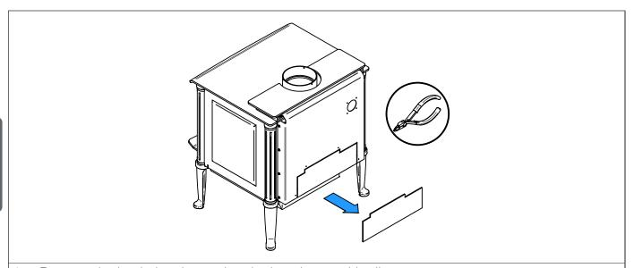
1. Remove the backplate by cutting the knockouts with pliers.
