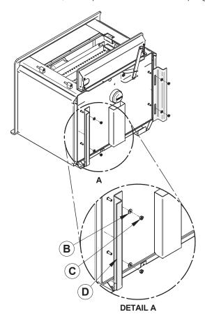
2. Put the stove on its back. Remove and dispose of the two freight supports **(D)**. Keep the nuts **(C)** and washers **(B)** for step 3.
