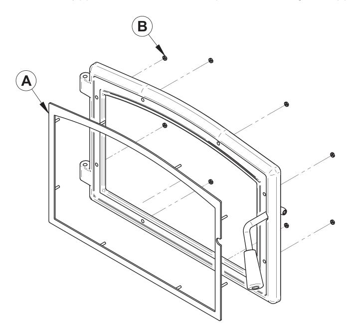
Note: It is not necessary to remove the glass to install the overlay.
