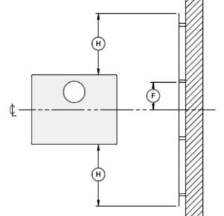
Figure 27: Heat shield clearances
