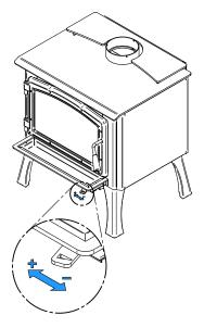
Figure 17: Air Supply Control
