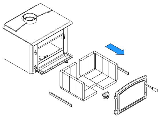
1. Remove the door, the firebricks, the spacers and the ash plug from the stove.
