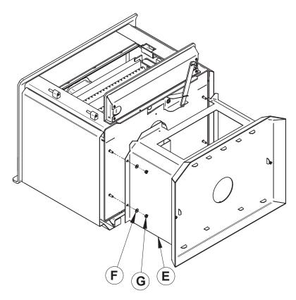
3. Install the pedestal **(E)** on the stove and screw it in place using the 4 the nuts **(G)** and washers **(F)** kept from step 2.
