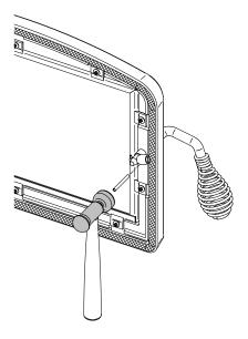
Figure 19: Installing the split pin
