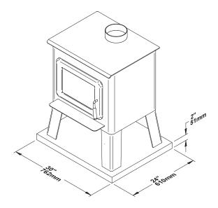
Figure 25: Floor protection for a mobile home
