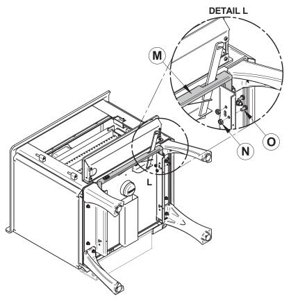
5. Install the molding (M) with the bolts (O) and nuts (N).
