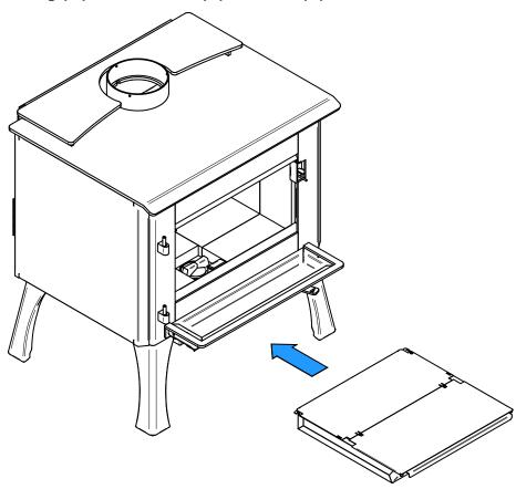
6. Put the stove on its legs and install the ash drawer included with the kit. Put back the firebricks, the spacers, the cast iron ash plug and the door on the stove. See step 1.
