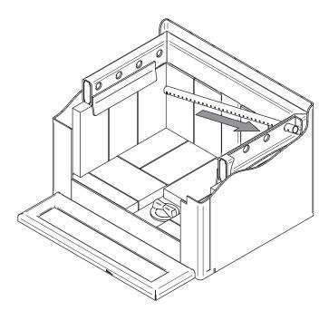
1. Starting with the rear tube, lean and stove the right end of the secondary air tube into the rear right channel hole. Then lift and stove the left end of the tube into the rear left channel.
