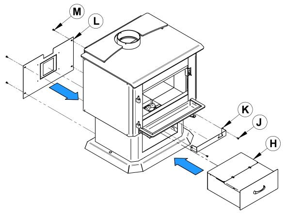
4. Put the stove on its pedestal and install the fresh air panel (L) with the screws (M), the molding (K) with the screws (J) and install the ash drawer (H). Put back the bricks, the spacers, the ash plug and the door on the stove. See step 1.
