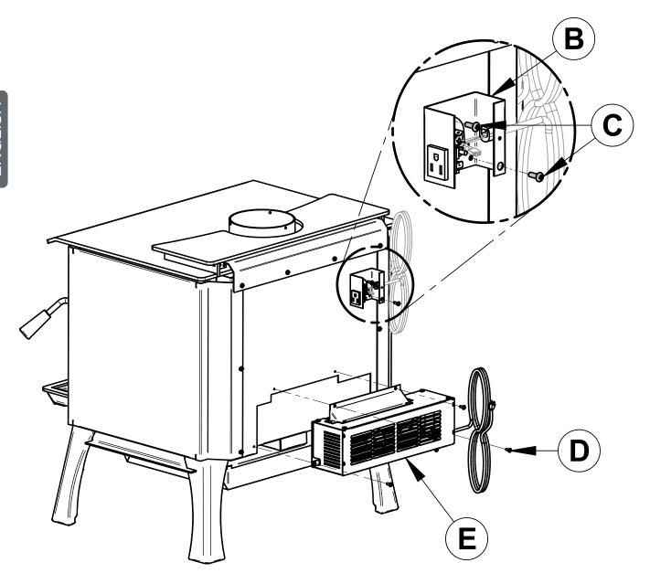
Screw the blower **(E)** into place using the screws **(D)** included in the installation manual. Screw the thermodisc **(B)** with the screws **(C)** supplied with the thermodisc on the back of the stove.
