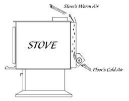
The blower is installed on the back of the stove to increase the flow of air past heat exchange surfaces and to help circulate warm air in the room. When used regularly, the blower can provide a small increase in efficiency, up to 2%. However, the use of a blower should not be used as a way to gain more output from a stove that is undersized for the space it is intended to heat.
