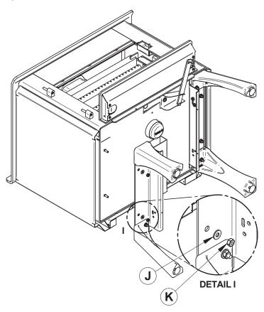
4. With the nuts (K) and washers (J) removed in step 1; secure both leg assemblies to the stove.
