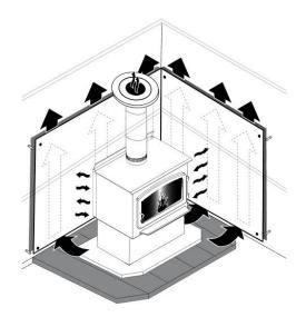
Figure 26: Heat shield
