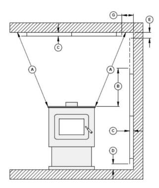
Figure 29: Heat shield clearances
