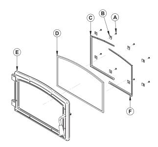
Figure 20: Replacing the glass
