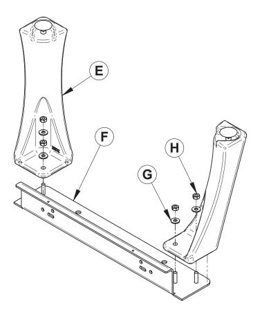
3. Install the legs **(E)** on the legs supports **(F)**. Secure with the washers **(G)** and nuts **(H)** supplied with the leg assembly.
