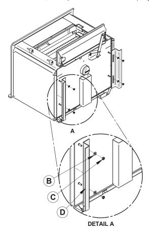
2. Put the stove on its back. Remove and dispose of the two freight supports **(D)**. Keep the nuts **(C)** and washers **(B)** for step 4.
