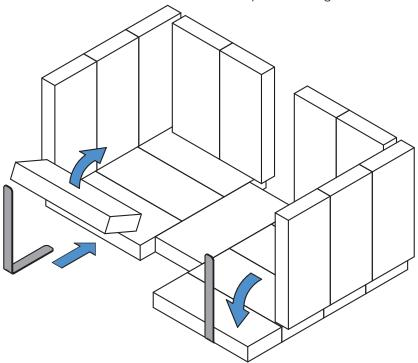
When installed, the log retainers can be adjusted side to side to support the first 2 inches of the end of a log when loaded in an East-West orientation (about 12» between the retainers).
