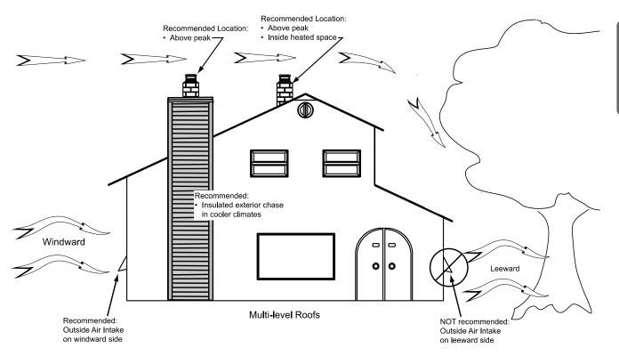
Figure 33: Air supply in conventional houses
