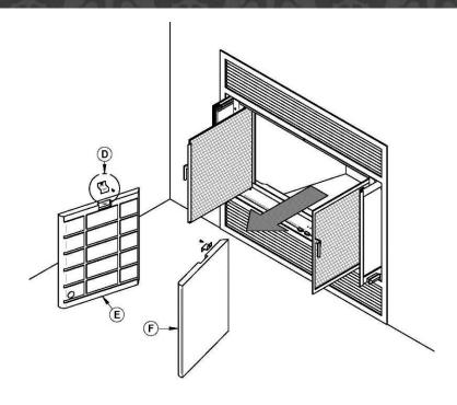
4- Remove the back refractory panel (G).
