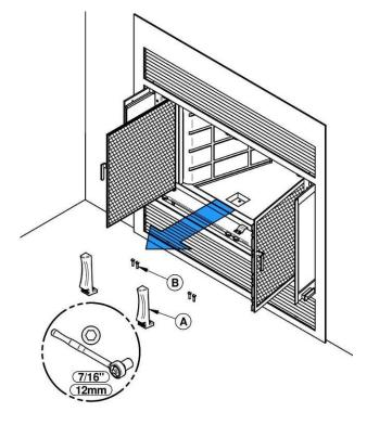
2- Remove the bottom refractory panel (C).
