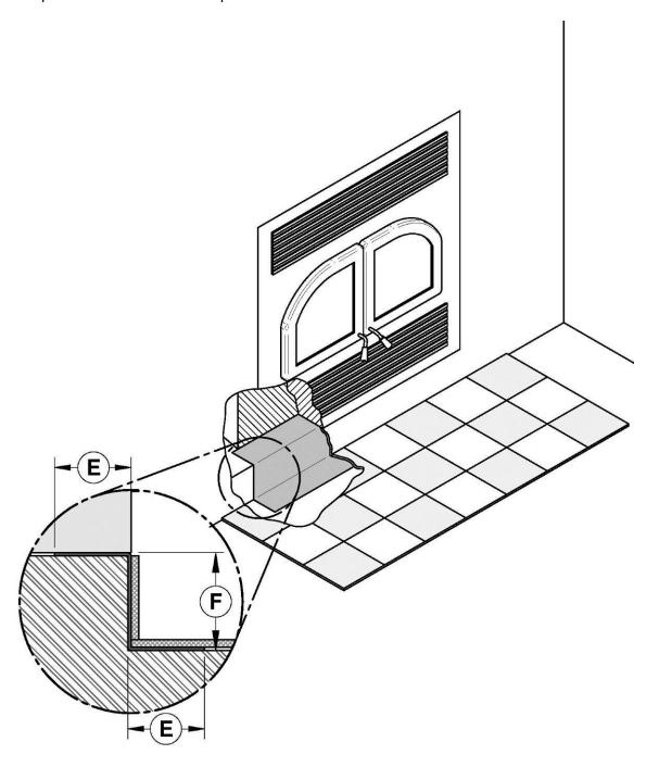
In the case where the fireplace is installed directly on the floor the joint between the hearth extension and the fireplace (E) must also be protected by a non-combustible material. For example, a sheet metal (not included).
