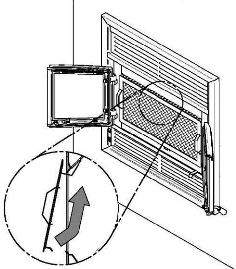
Lean the upper part of the firescreen against the top door opening making sure to insert the top firescreen bracket behind the primary air deflector as in (DETAIL A).
