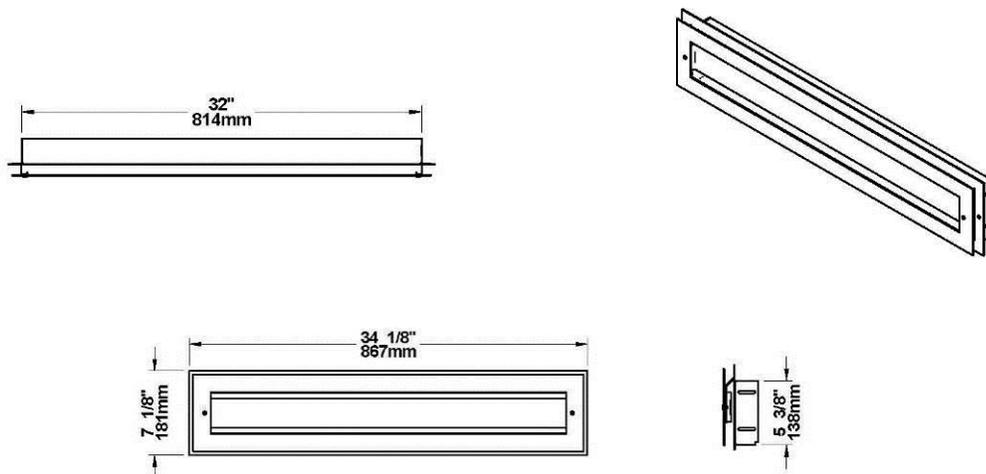
**DIMENSIONS OF ASSEMBLED HEAT DISTRIBUTION BOX AND ADJUSTABLE DECORATIVE PLATE:**
