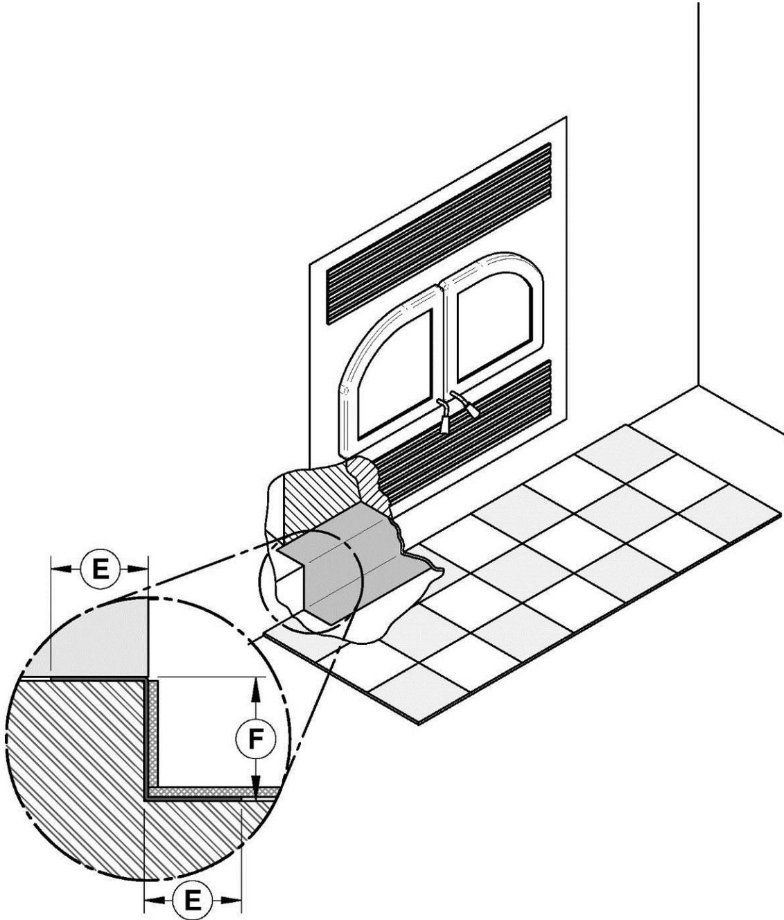
**6.3.1.2 On the floor or on a raised base of less than 4" installation (R value for the hearth extension required)**
