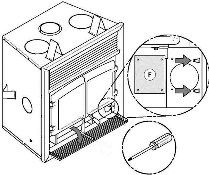
Flip the fireplace's lower decorative louver. Install the blocking plate (F) included in the kit, on the front opening of the air control housing. Using a screwdriver, secure with two screws.
