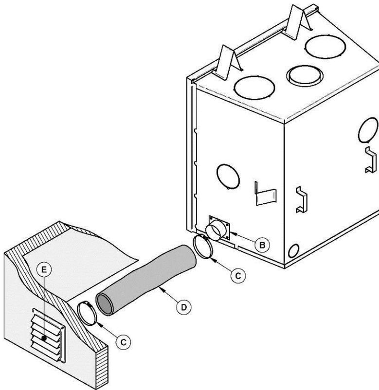
Then, install the flexible pipe\* (D) (not supplied) to the fresh air intake adapter (B) using one of the adjustable pipe clamps (C). Secure the other end of the pipe to the outside wall termination (E) using the second adjustable pipe clamp (C). The outside wall termination (E) must be installed outside of the building.
