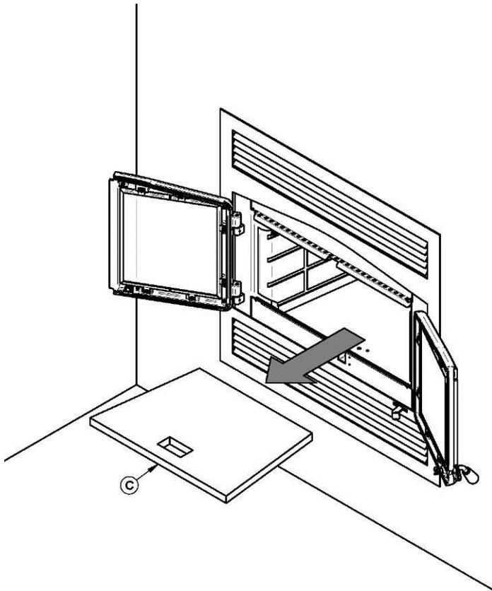
2. Remove the floor refractory slab (C).
