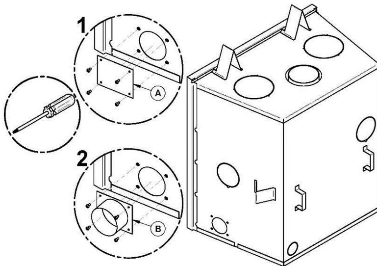
**(1)** Using a Philips screwdriver, remove the four screws holding the rectangular plate **(A)** on the right of the fireplace jacket. If the location 2 or 3 has been chosen, use pliers to remove the knock-out.
