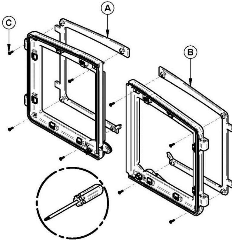
Position the overlays (A) and (B) on the door frames and secure them from the inside of the doors using the 8 included screws (C).
