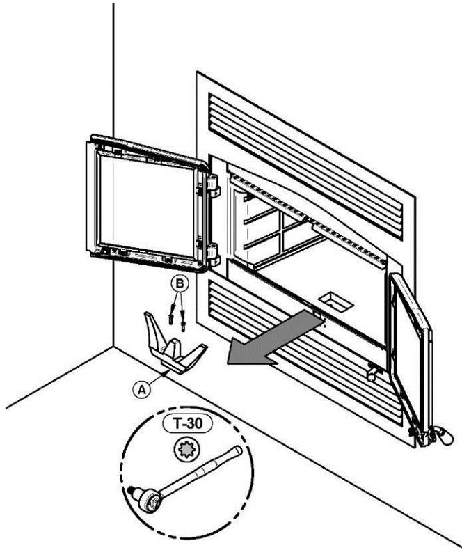
1. Using a ratchet key and a Torx (T-30), unscrew the two Torx screws (B) holding up the andiron (A).
