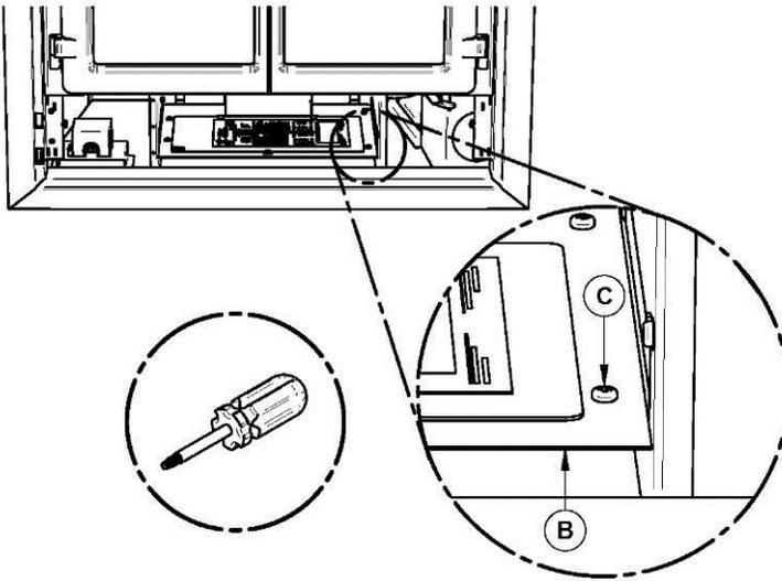
3. Remove and keep the heat shield (B) and the 4 screws (C).
