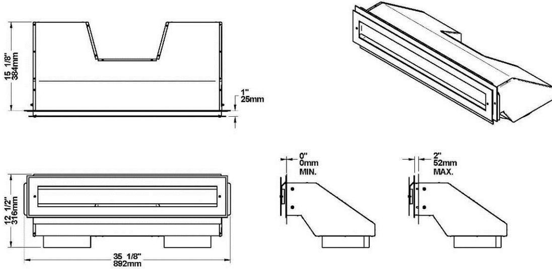
**DIMENSIONS OF TELESCOPING SECTION**
