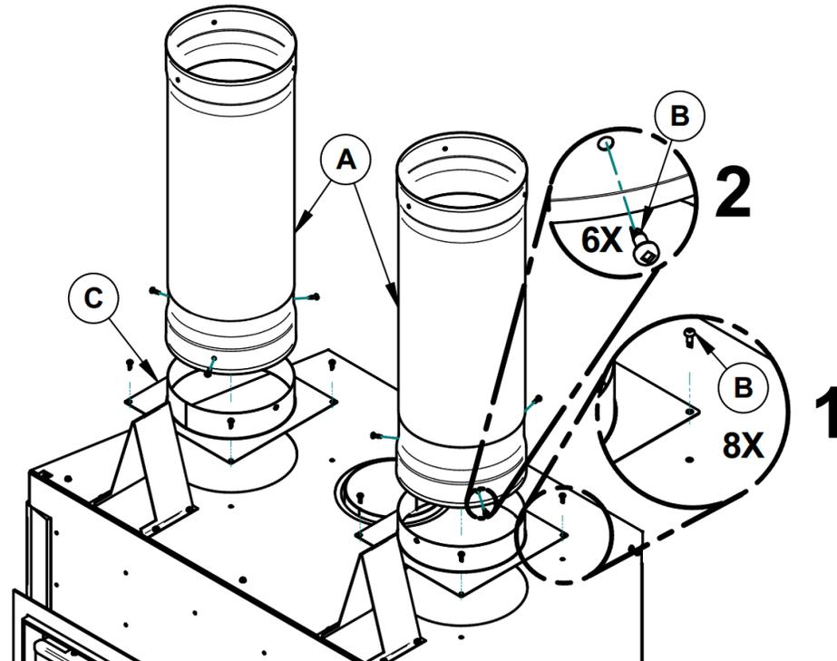
Secure the telescoping sections (A) to the heat distribution box (C) with self-tapping screws (B) (3 per telescoping section). Determine the needed height and secure the two parts of the telescoping sections together with 3 self-tapping screws provided. Insert the adjustable frame (D) in the heat distribution box (C), press it against the non-combustible finishing material and secure with 4 screws into the heat distribution box. Set the decorative plate (E) to the adjustable frame (D).
