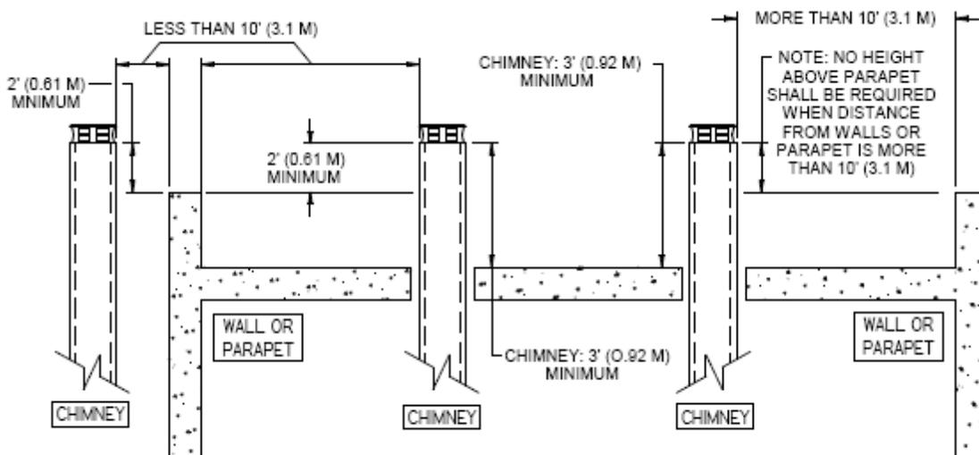
12. For installations where more than one chimney is located in the same non-chase or within the same area, we suggest that their terminations be separated by at least 16" (410 mm) horizontally, and 18" (460 mm) vertically. This separation is to prevent smoke migrating from one chimney to another.
