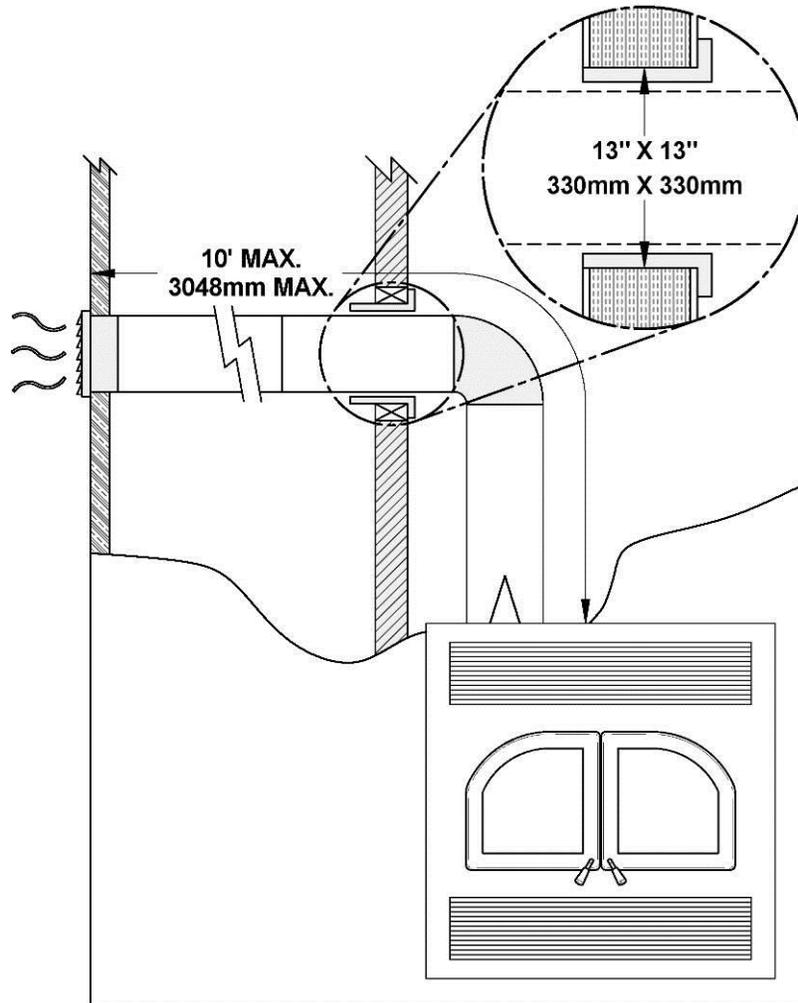
8. Do not connect the hot air ducts to a central heating system. Malfunction of the heating system's fan will cause the fireplace to overheat.
