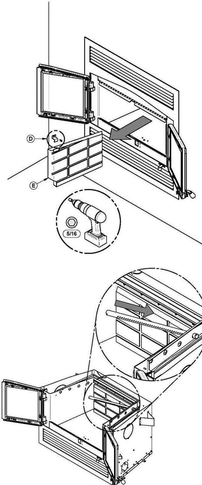
3. Using a power screwdriver and hex tip 5/16", remove the slab holder (D) and the left refractory slab (E).
