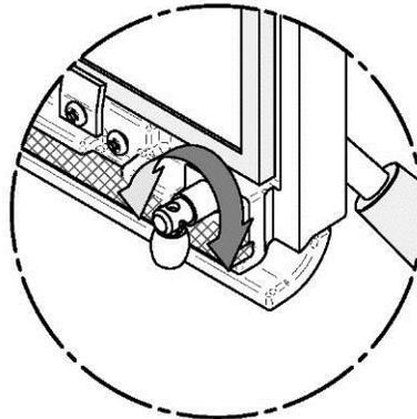
3. Re-install the split pin with a small hammer.
