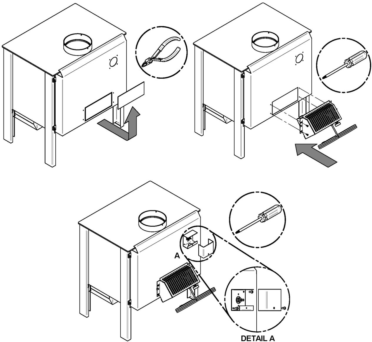
When using the optional blower, allow the stove to reach operating temperature (approximately one hour), before turning it on. The increased airflow from the blower cools the firebox and could affect the start-up combustion efficiency if the blower is turned on too early. You can also install a thermodisc to enable the blower to start or stop automatically when the stove is hot or too cold. The thermodisc part number is AC05530 for a basic model and ACO2055 for a quick connect model.
