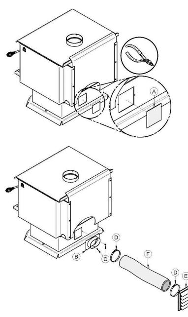
Remove the disposable metal plate (A) behind the pedestal using a pair of pliers.
