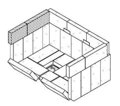
1. Remove the top left bricks as shown in picture.
