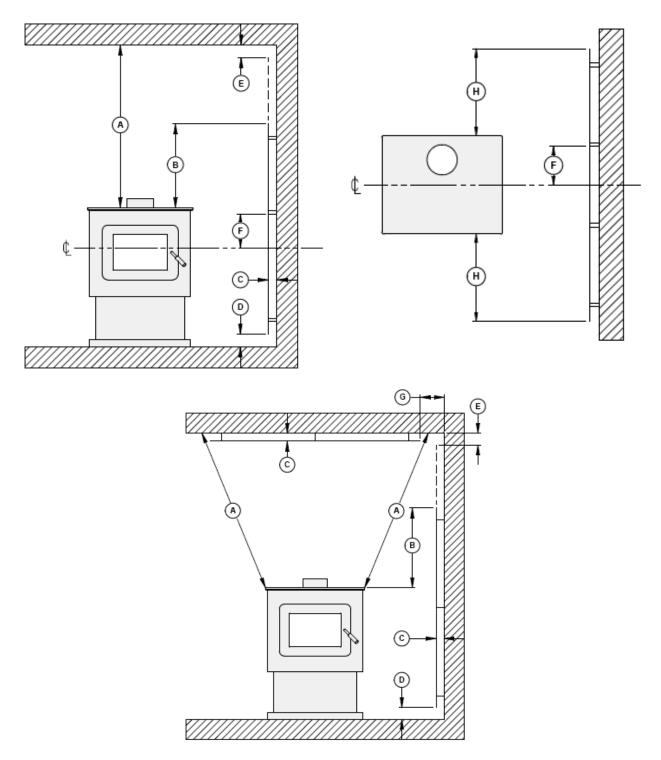
**Clearances for shield construction**
