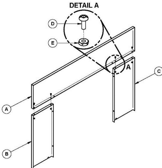
Line up the holes of the upper faceplate panel (A) with the holes of the side panels (B) and (C). Secure them together using four (4) bolts (D) and nuts (E) provided (see **DETAIL A**).
