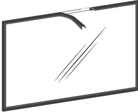
Do not abuse the glass door by striking or slamming shut. Do not use the insert if the glass is broken. To change the glass, perform the same operation described above.
