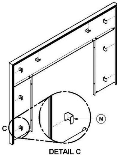
Secure the trim to the faceplate by squeezing the eight trim retainers (M) between the inner edge of the trim and the front of the faceplate. As in the image on the left.
