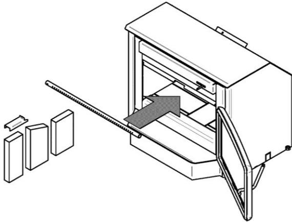
9. Replace the secondary air tube followed by bricks and brick bracket removed in **Step 1**.
