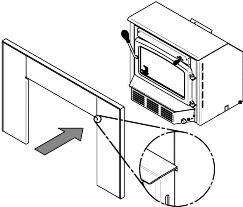
Center the insert into the fireplace opening. Adjust its height using the leveling bolts on each side of the convection air jacket box until the faceplate is properly seated on the floor of the hearth extension.
