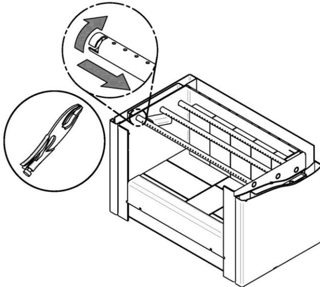
2. To remove the secondary air tube, hold it with a pair of pliers and follow the movement described.
