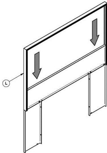
Align the trim assembly (L) with the left and right edge of the faceplate and slowly slide it down over the faceplate.
