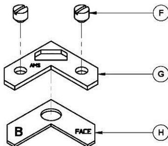
Partially thread the screws (F) on the trim's corner bracket (G) then superimpose the corner brackets (G) and (H) as shown in the image on the left.
