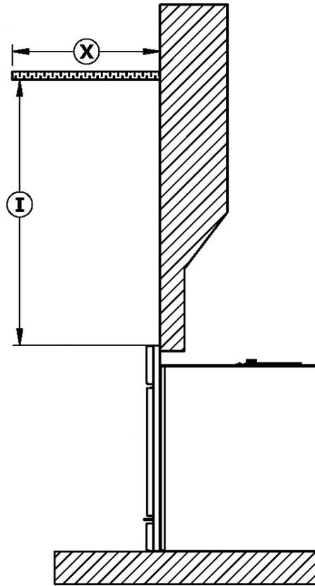
Note that you can reduce the mantel shelf clearance with the use of a heat shield, as described below.
