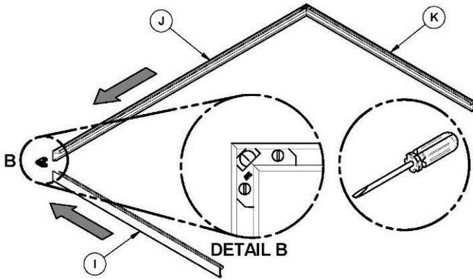
Insert the superimposed brackets (G) and (H) with the screws (F) in the groove of each decorative trim (I), (J) and (K) (see **DETAIL B**). Align the corners of the angled side of each trim, and then tighten the screws (F) to secure the trims.
