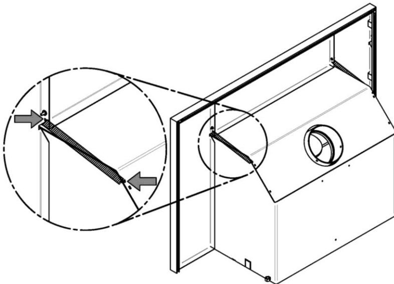
Then install one faceplate retainer spring on each side of the faceplate and attach the other end of the spring to the holes in the slanted part on the left and right sides of the of the convection air jacket as shown in **DETAIL B**.
