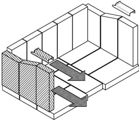
1. Remove from the firebox the hatched bricks (3) and left bricks retainer as shown in the diagram.
