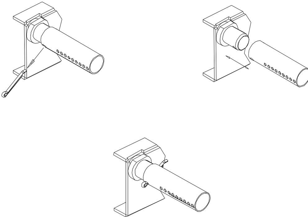
**Figure 4.3 – Secondary Air Tube replacement**
